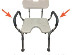
Place the chair upright so that it is resting evenly on all four legs and insert the arms into the frame. Depress both push buttons and push down until the push buttons "click" and lock into position. Repeat this step for the opposite arm.
