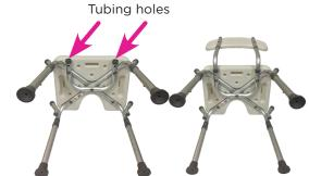
Turn the chair on its side so that the tubing holes are facing upward. Insert backrest into tubing holes until the push buttons "click" and lock into position.
